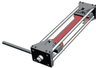
Figure 6: Uniaxial test rig (load applied by torque wrench)
